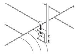
Screw the bracket to the edge of the table top.
